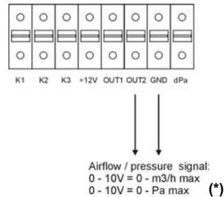
(\*NL: Maximaler Outputstrom = 10 mA. Maximale Output Impedanz = 50 kΩ.
